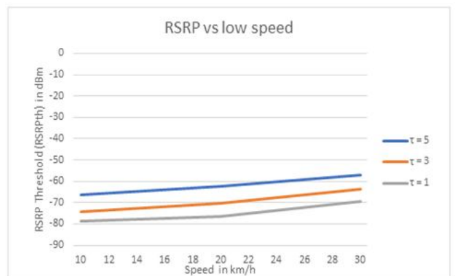
Figure 6: RSRP Threshold for Low Speed UE with Different \tau
