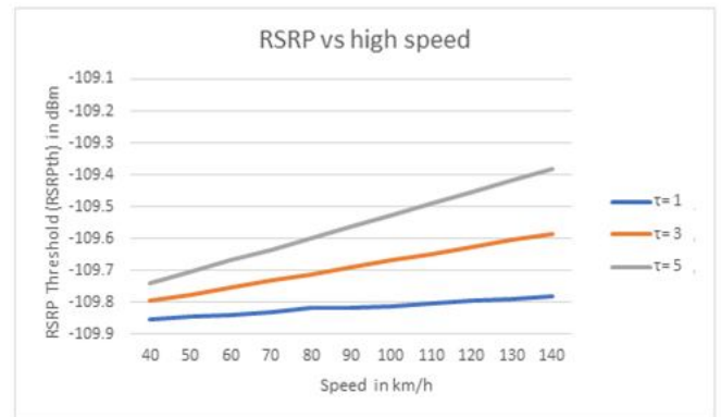
Figure 5: RSRP Threshold for High Speed UE with Different \tau
