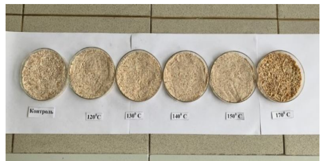
Figure 3: Protein fillings when dried at different temperatures (120-1700 C)
