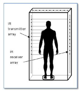
Figure 4: IR Transmitter and IR Receiver Array for Mechanical Assembly
