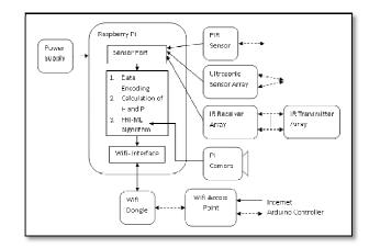
Figure 8: Entry Gate System using Raspberry Pi Controller
