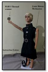
Figure 19: Humanoid Robot Model for Scanning with Thermal Camera
