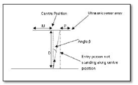
**Figure 7b:** Geometry for Calculation of Angle  $\beta$  (top view)
