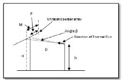
**Figure 7a:** Geometry for Calculation of Angle  $\beta$  (side view)
