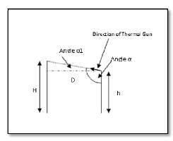
Figure 6: Geometry for Calculation of Angle  $\alpha$
