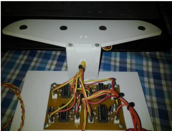
Figure 6: The actual hardware set-up for the four microphones.
