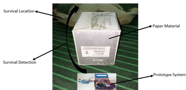
Figure 15. Aliveness detection under paper bundle
