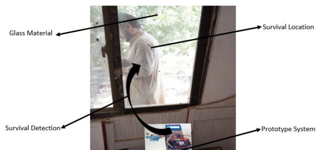
Figure 14. Aliveness detection behind glass structure
