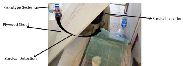
Figure 13. Aliveness detection through Plywood structure
