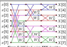
Figure 5: DIF for 8-points FFT algorithm.
