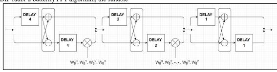
Figure 6:System model for simple 8-points FFT processor.
