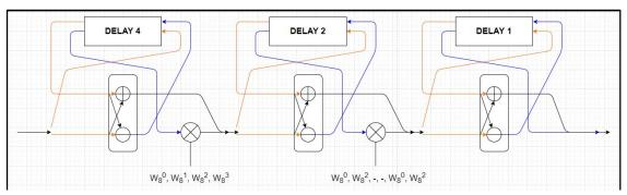
Figure 7:System model for single-path delay feedback 8-points FFT processor.
