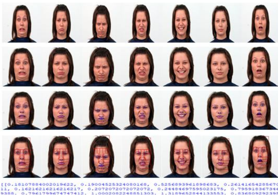
Figure5. The process of our FSR, line1: extract of the dataset photos/input facial emotion. Line2: cropped emotional photos. line3: extract the 68 face landmarks points. Line 4: calculate of sixteen features and line5: the vector generated from the facial emotion photos, it is involved to recognized the kind of emotion. The output result of FER is the probe kind of emotion of the input facial photos
