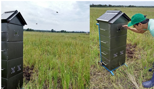
Figure 6: Actual rice field soil data collection using Solar-powered soil nutrient detector device
