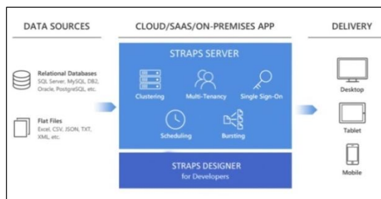
Figure 3: Cloud Computing (SaaS) Architecture for STRAPS
