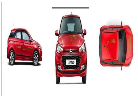
Figure 7: The detected dents and the scratches of all the views in a single image
