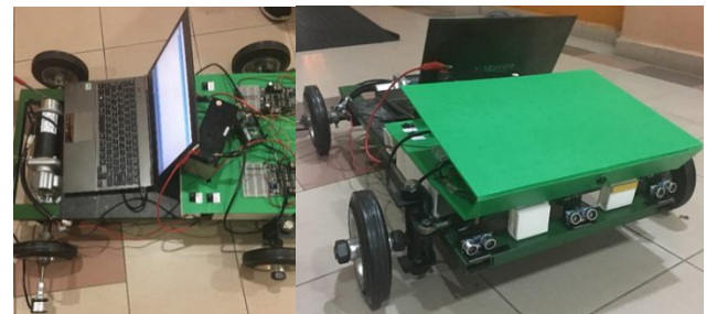
Figure 8: Prototype of Cart Follower
