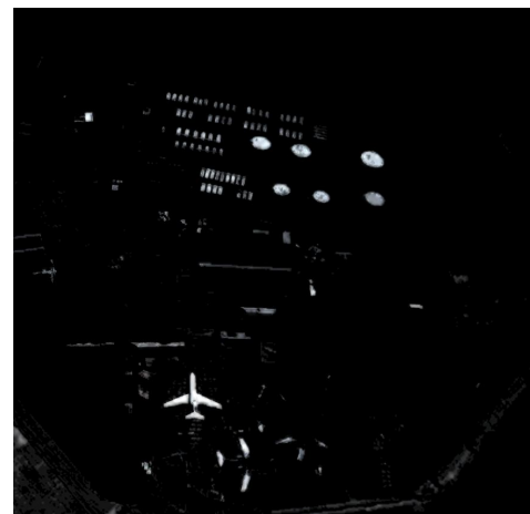
Figure 8: The rescale The determining of the resulting image fs_r(X) – pixelwise product of image f_{K_1}(X) and the image-filter f_i(X) by expression (4)
