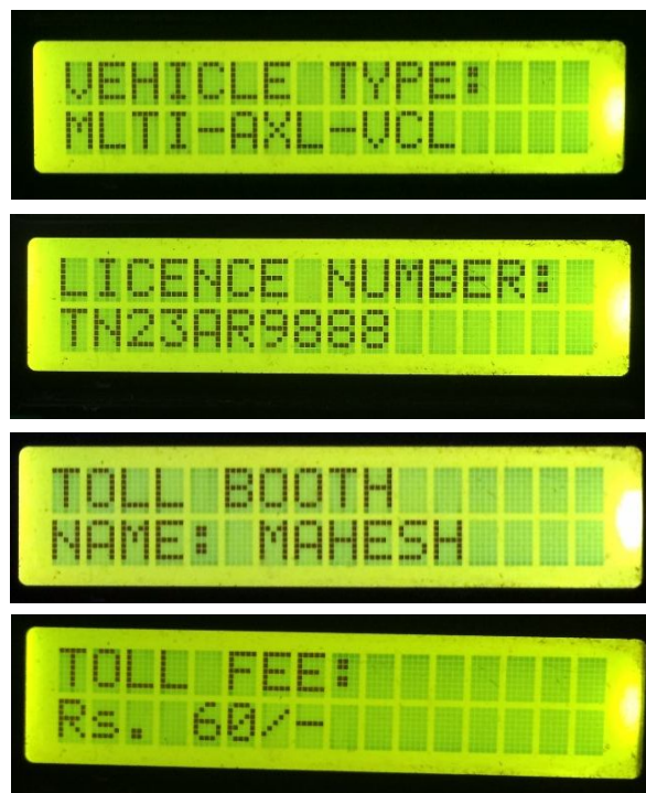
Figure 13: -Displaying The Details of The Driver on Liquid Crystal Display
