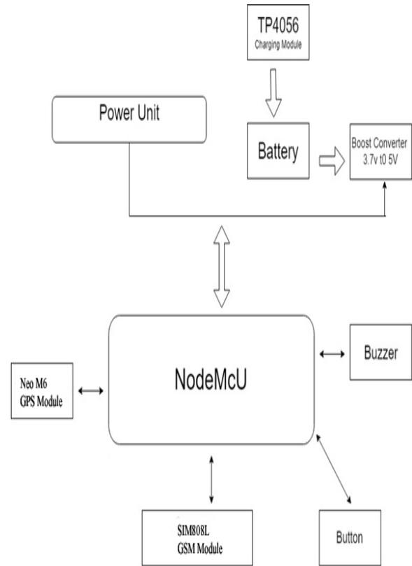
**Figure 5.1:** Hardware Selection Working Flow.
