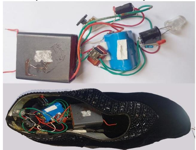
**Figure 5.2:** Electric Shock Generator with Sandal
