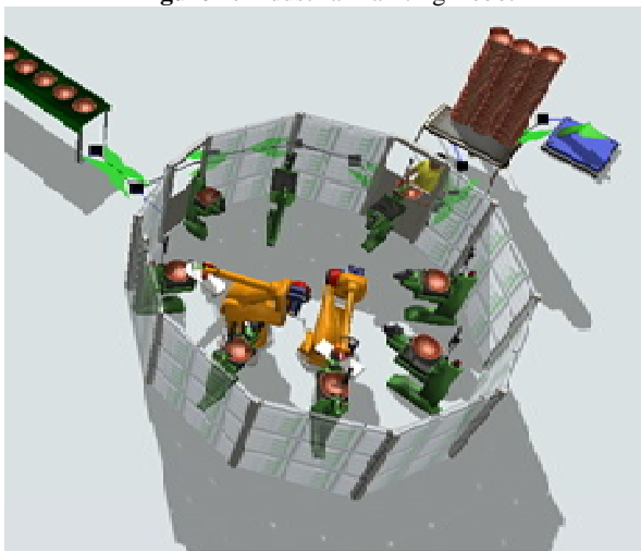
Figure 2: Simulation of the Robots installed in Painting Station
