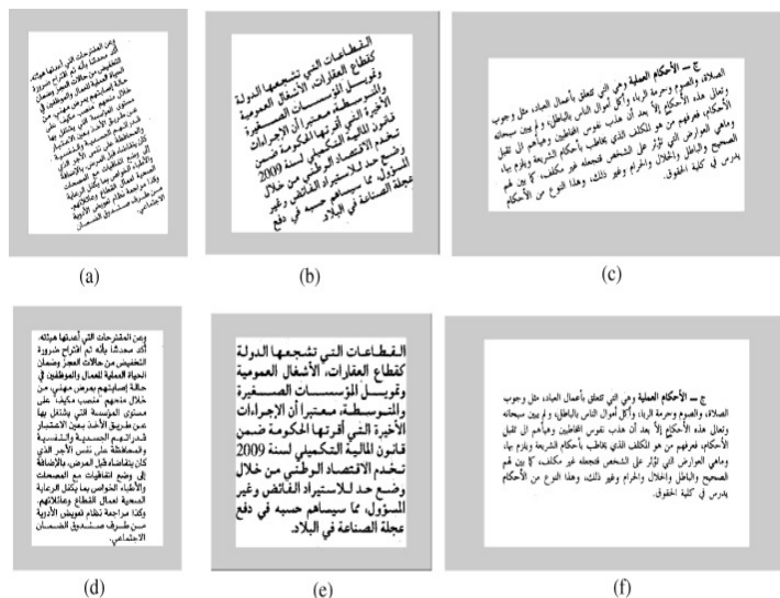
Figure 7. (a,b) images of skewed document from Algerian newspapers; (c) image of skewed document from Arabic book.;(d, e, f) images of skew-corrected document of the images (a, b, c) correspondingly
