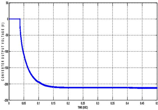
**Figure 17(a):** Buck Boost converter output voltage
