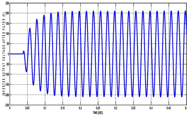
**Figure 21:** Inverter output voltage after filter
