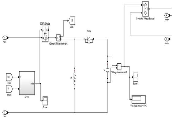
**Figure 7:** Simulink model of Buck Boost converter with INC MPPT method
