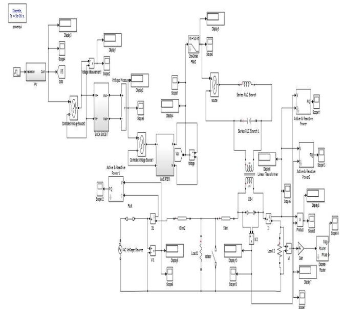
**Figure 10:** Simulink model of the overall test system with R load
