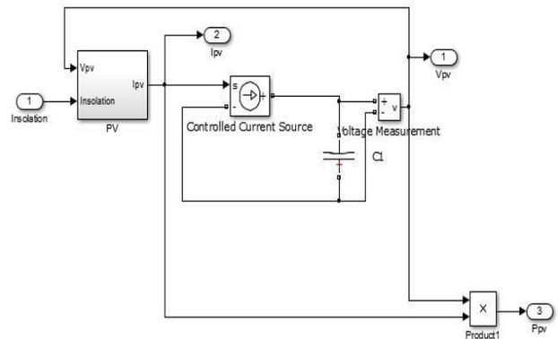
**Figure 6:** Simulink model of solar PV module
