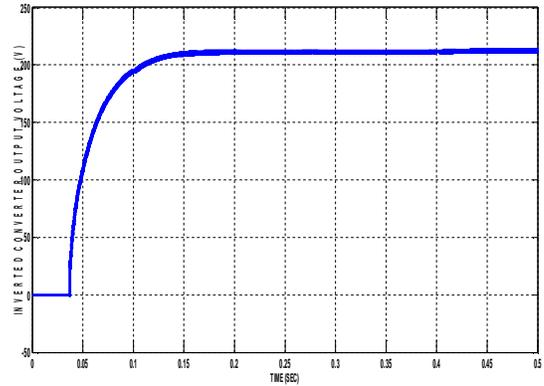
**Figure 18 (a):** Inverted Buck Boost converter output voltage
