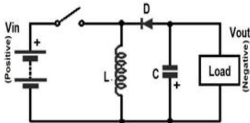
**Figure5:** DC-DC Buck Boost Converter (negative type)[1]
