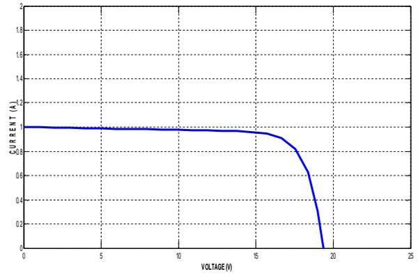
**Figure 13:** I-V characteristics of PV module
