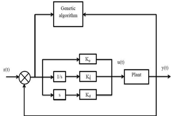
**Figure 3:** Structure of GA-PID controller[4]
