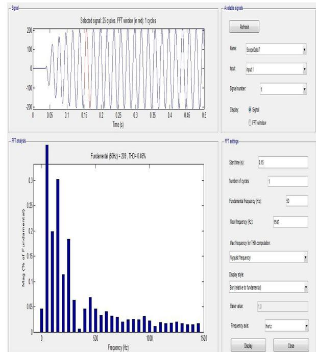
**Figure 35:** FFT analysis showing percentage of the harmonics
