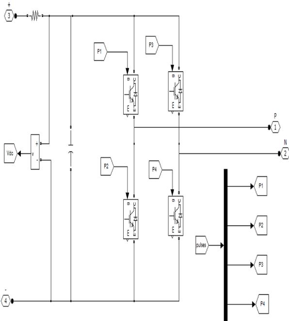
**Figure 8:** Simulink model of single phase inverter
