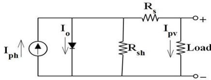
**Figure 2:** Single diode equivalent circuit of a solar PV cell [1]
