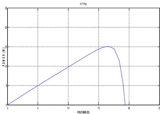
**Figure 12:** P-V characteristics of PV module
