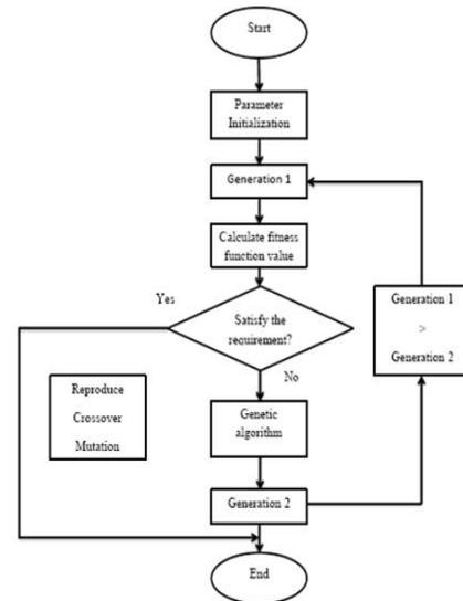
**Figure 4:**Flow-chart for auto tuning GA-PID controller [2]
