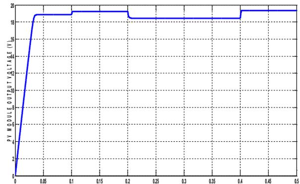
**Figure 15:** PV module output voltage with variable insolation
