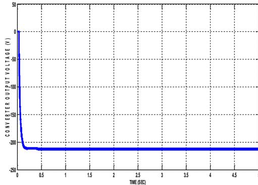
**Figure 17. (b):** Buck Boost converter output voltage
