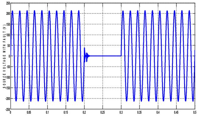
**Figure 23:** Source voltage with fault
