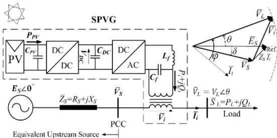
**Figure 1:** Schematic diagram of the SPVG interconnected to a grid system [1]
