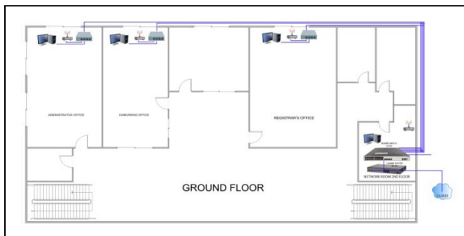
Figure 1: Physical network design ground floor.
