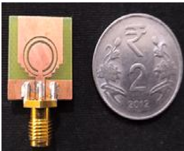
Figure 8: Prototype of the dual notch band antenna.
