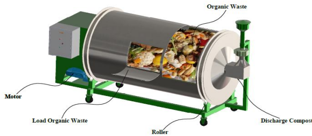
Figure 1: Movement of materials in the industrial rotary composter
