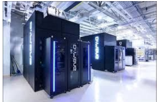
Figure 5.7 - Using the SQUID as the building block, D-Wave systems has built the Quantum computer which looks as this
