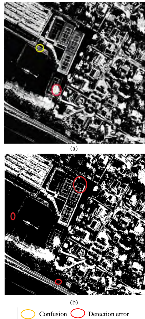
Figure 6: Visual interpretation of the best results by (a) ISOFAP and (b) PCA-K-means on images 1.
