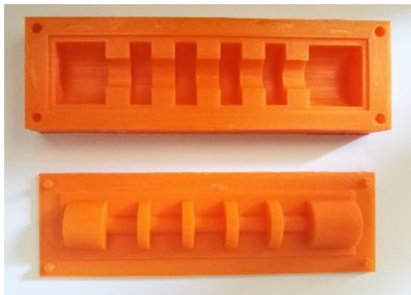
Figure 3: The 3D printed mould; (a) bellow side outer layer (b) bellow side inner layer
