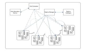
Figure 4: global model of centralized job scheduling and replication
