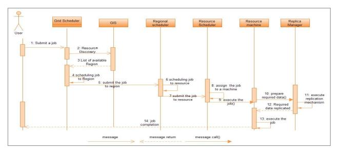
Figure 2: sequence Diagram of hierarchical job scheduling
