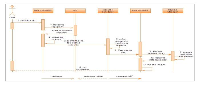
Figure 1: Sequence Diagram of centralized job scheduling
