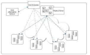
Figure 3: Structure of centralized job scheduling and data replication
