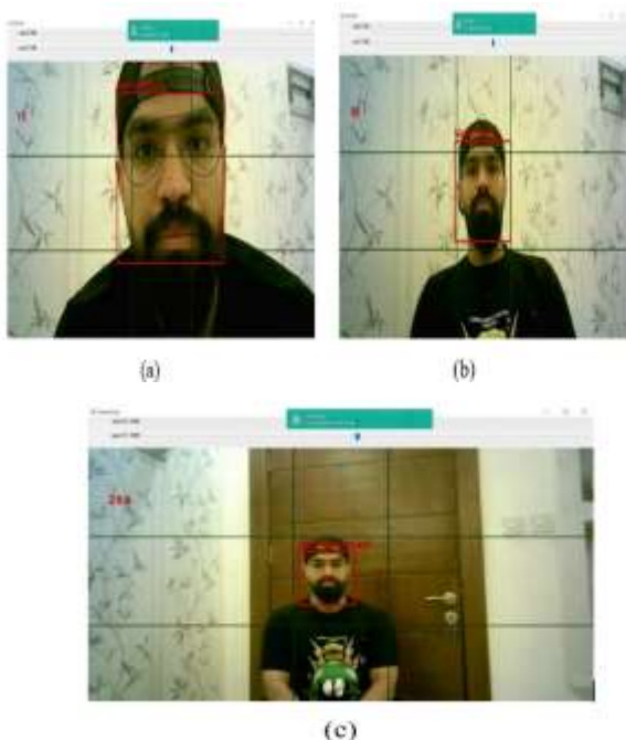
Figure 9: (a) Person is 0.5 meter away ,(b) Person is 1.5 meter away, (c) Person is 2.5 meter away
