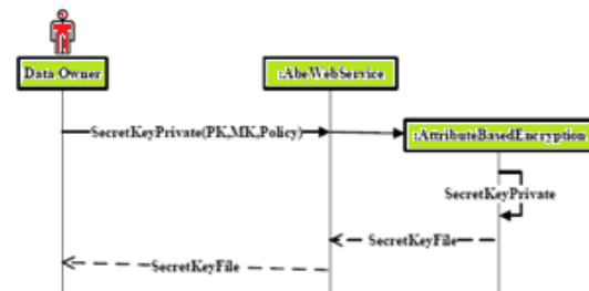
Fig. 3 - Sequence Diagram for the Set-Up for Personal Domain User
