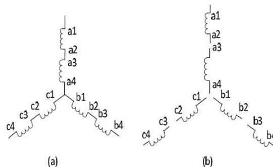
Fig. 4 Induction Motor stator winding: (a) General arrangement (b) Arrangement for the proposed inverter
