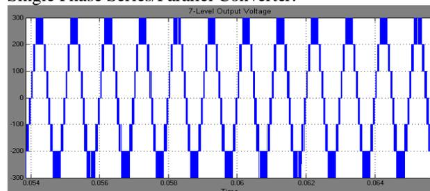
Fig. 6 Seven Level Output Voltage
