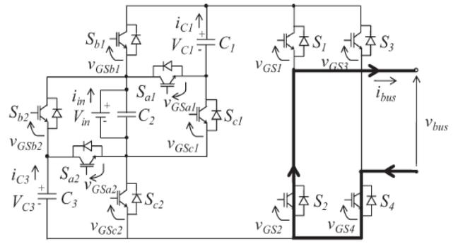
(a) The current  $i_{bus}$  does not flow in the capacitors  $C_k$ .
