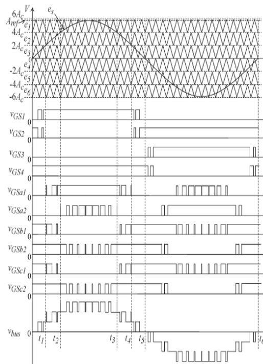
Fig. 3. Modulation method of the proposed inverter ( $n = 2$ ).
