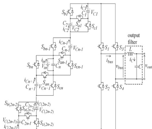
Fig.1. Circuit topology of the switched-capacitor inverter using series/parallel conversion
