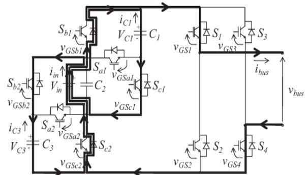
(b) All capacitors are connected in Parallel
