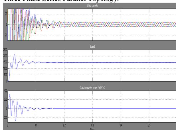
Fig.12 Stator Currents, Speed, Electromagnetic Torque of Proposed Three Phase Series/Parallel Topology Applied to Induction machine Drive.
