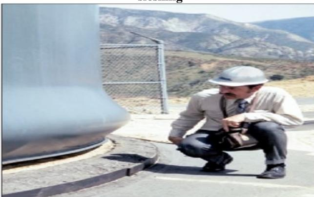
**Figure 2.3: Elephant-foot buckling of a tank wall**
