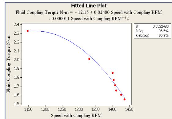
**Fig 11:** Fitted Line plot for Output disk torque
