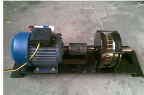
**Fig 2.** Induction motor with fluid coupling
