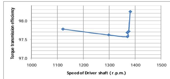
Fig 6: Variation of torque transmission efficiency with speed of driver shaft
