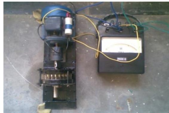
**Fig 4.** Wattmeter connected to motor
