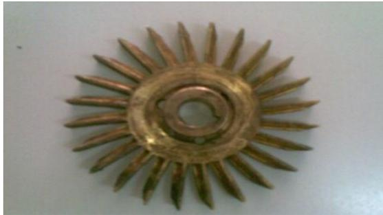
Fig 5. Impeller of pump and turbine
