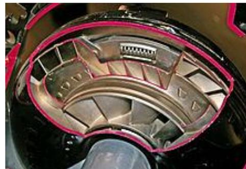
**Fig 1.** Torque Converter
