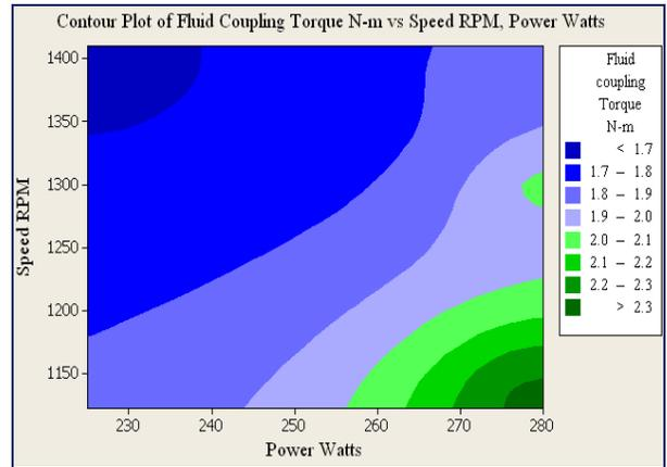
**Fig 10:** Contour plots of Output disk torque
