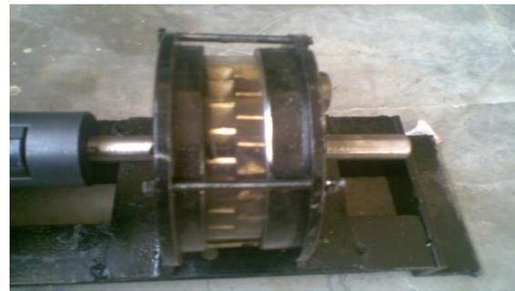
**Fig 3.** Fluid coupling
