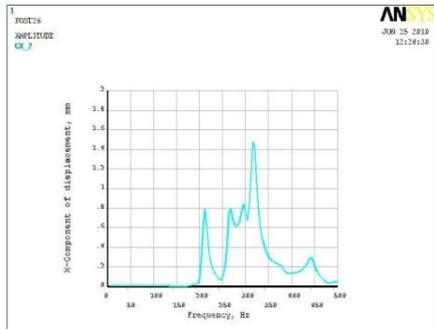
**4.3.5 X-Y-Z Component of Displacement versus Frequency response graph of Composite blower**
