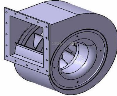
**Fig. 3.1.1 Solid model of the centrifugal blower**
