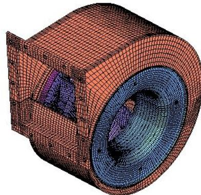
**Fig.3.2.1 Centrifugal Blower FE model in Hypermesh 10.0**
