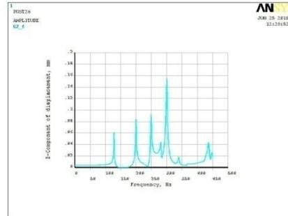
4.3.4 X-Y-Z Component of Displacement versus Frequency response graph of aluminum blower
