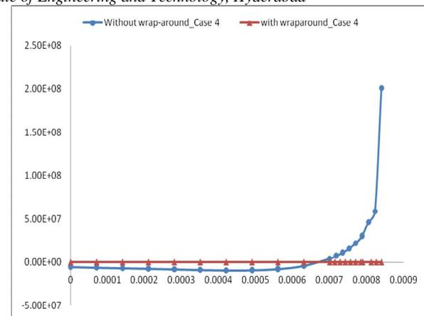
Figure 36: Distribution of the interlaminar normal Stresses along width case 4
