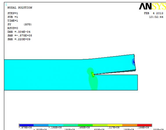
Figure 22: Contour of normal stress Delaminated model without wrap around case 2
