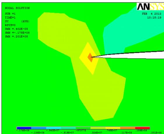
Figure 20: Variation of normal stress around the crack tip delaminated model with wrap-around Case 1
