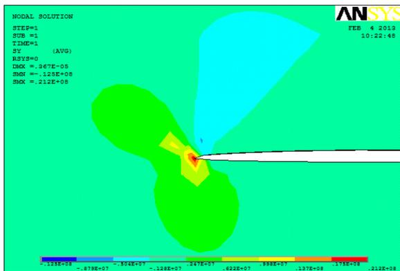
Figure 25: Variation of normal stress around the crack tip delaminated model with wrap-around Case 2
