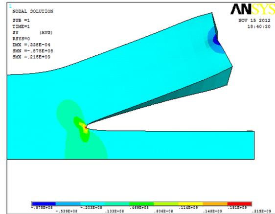
Figure 17: Contour of normal stress Delaminated model without wrap around case 1
