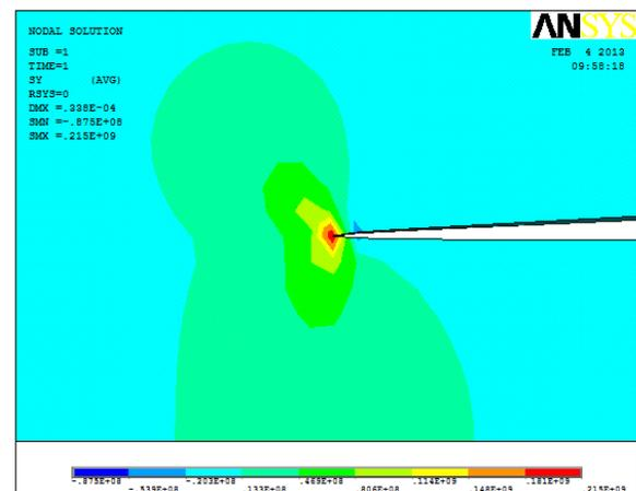
Figure 18: Variation of normal stress around the crack tip delaminated model without wrap-around Case 1
