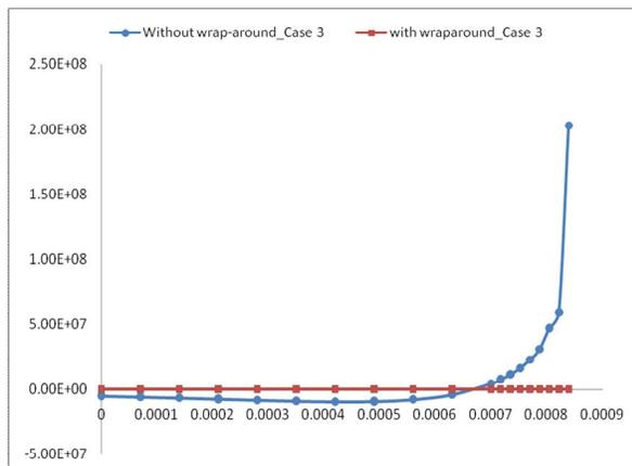
Figure 31: Distribution of the interlaminar normal Stresses along width case 3
