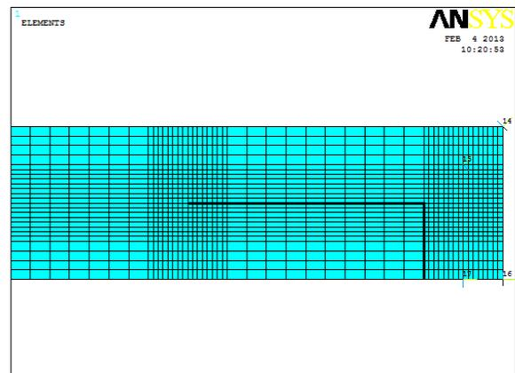
Figure 12: Mesh distribution with wrap-around case 2
