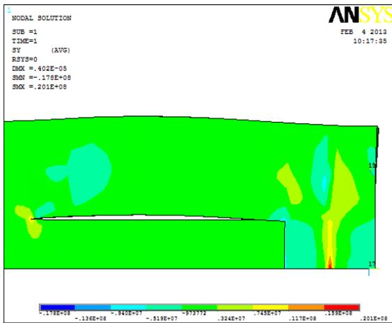
Figure 19: Contour of normal stress Delaminated model with wrap around Case 1
