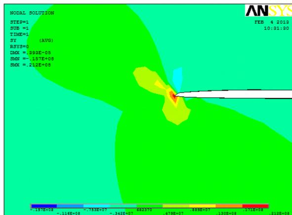
Figure 35: Variation of normal stress around the crack tip delaminated model with wrap-around Case 4
