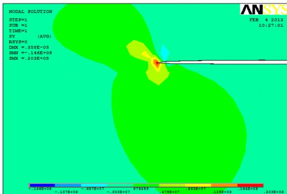
Figure 30: Variation of normal stress around the crack tip delaminated model with wrap-around Case 3
