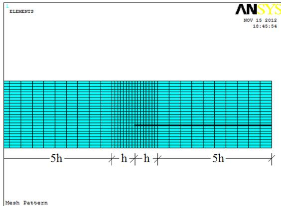
Figure 9: Mesh distribution without wrap-around Case 1
