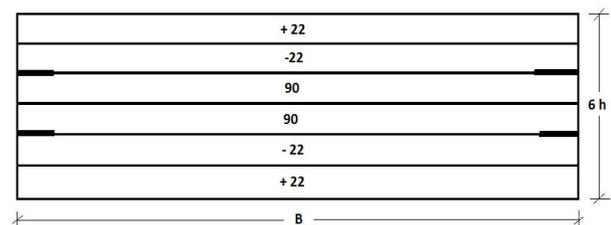
Figure 5: Delaminated model without wrap-around (+22/-22/90)<sub>s</sub>
