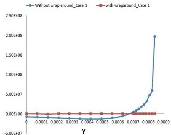
Figure 21: Distribution of the interlaminar normal Stresses along width case 1
