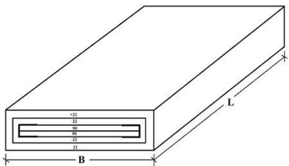
Figure 7: Delaminated model with wrap-around (+22/-22/90)
