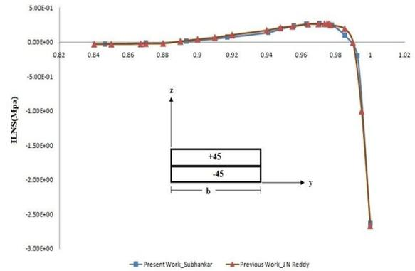
Figure 4: Comparison of ILNS ( $\sigma_z$ ) distribution across width(y/b) at laminate interface
