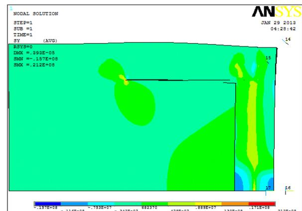
Figure 34: Contour of normal stress Delaminated model with wrap around Case 4
