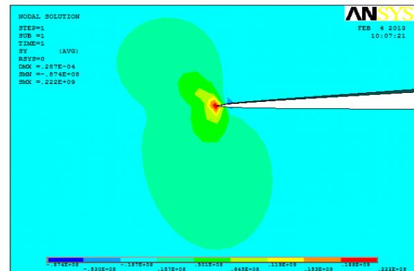
Figure 28: Variation of normal stress around the crack tip delaminated model without wrap-around Case 3
