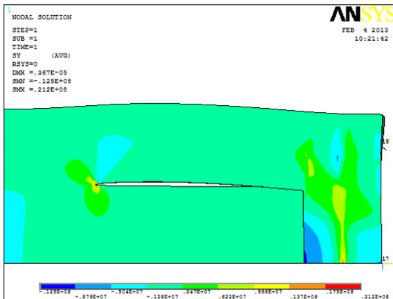
Figure 24: Contour of normal stress Delaminated model with wrap around Case 2
