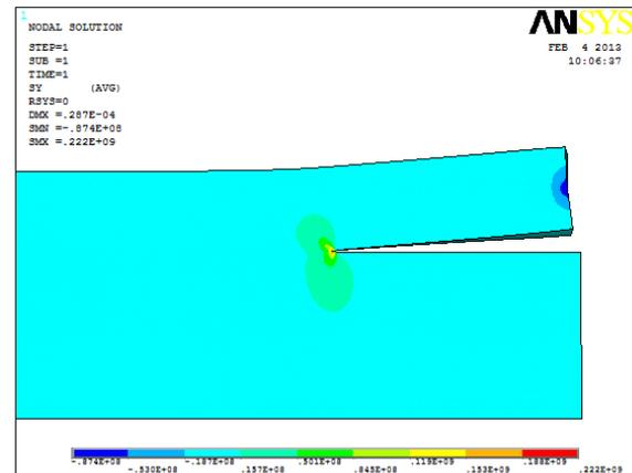
Figure 27: Contour of normal stress Delaminated model without wrap around case 3
