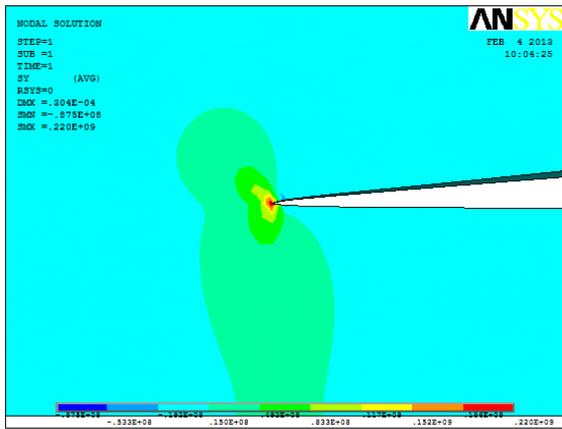
Figure 23: Variation of normal stress around the crack tip delaminated model without wrap-around Case 2
