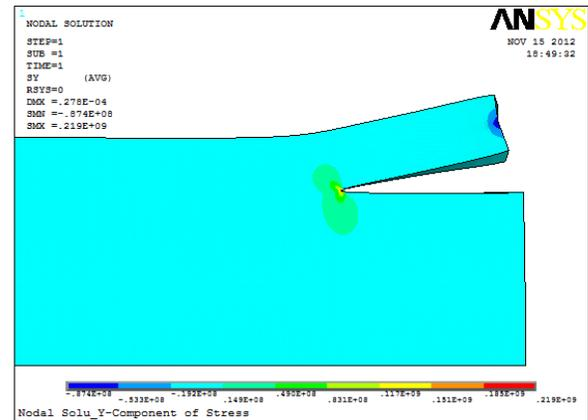
Figure 32: Contour of normal stress Delaminated model without wrap around case 4
