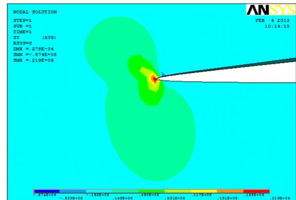
Figure 33: Variation of normal stress around the crack tip delaminated model without wrap-around Case 4
