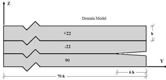
Figure 6: One fourth model without wrap-around
