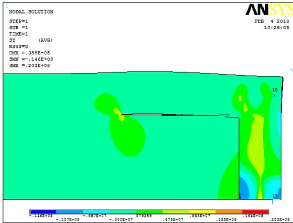
Figure 29: Contour of normal stress Delaminated model with wrap around Case 3
