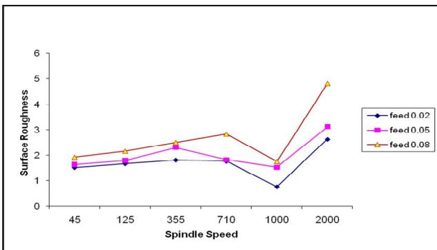
Fig. 2 (a) - 4mm φ Drill and different Feed Rates
