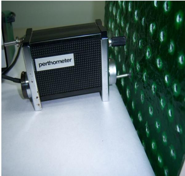
Fig: 1: Analysing surface roughness by Perthometer
