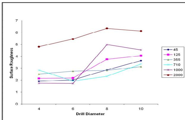
Fig 3 (c) – 0.08 mm/rev Feed Rate and different Spindle Speeds
