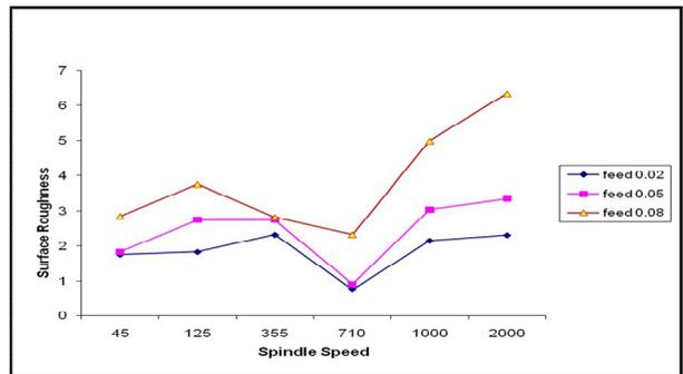
Fig 2 (c) – 8mm φ Drill and different Feed Rates
