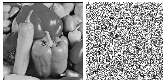
(a) Original image (256 x 256) (b) Segmentation of gradient image without median filter and thresholding
