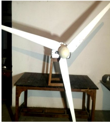
Figure 19: The complete assembly of wind turbine
