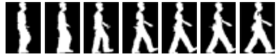
Figure 1. Background subtraction normalized and aligned silhouettes of a gait cycles from a gait sequence.
