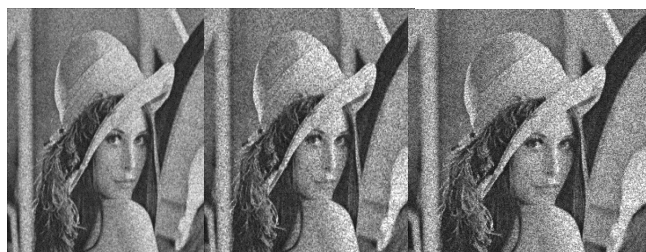
Figure.7 (a) Speckle noise Removal with mean Filter. Figure.7 (b) Speckle noise Removal with median Filter. Figure.7(c) Speckle noise Removal with adaptive Median Filter
