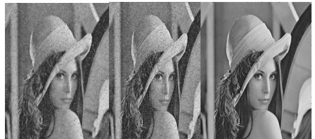
Figure 1 (d): Salt and Pepper Noise Removal with Weiner Filter. Figure.1 (e) {Salt and Pepper removal with Average Filter. Figure1 (f) { Salt and Pepper removal with median Filter.
