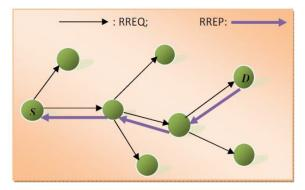
Figure 2: AODV routing protocol with RREQ and RREP message
