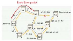
Figure 6: Building of the route record during route discovery
