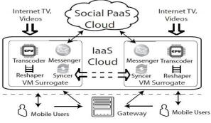
Figure 4: Architecture of Cloud MOV
