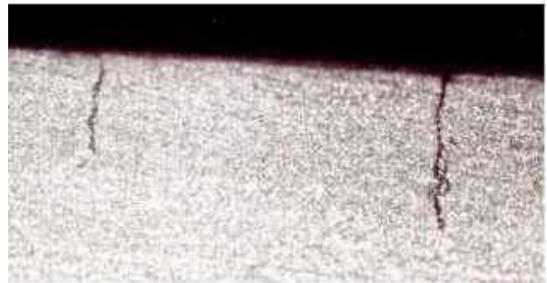
Figure 2: Picture showing a crack in an oil pipe
