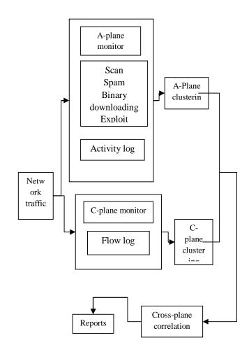
Figure 3. Architecture of Bot Miner
