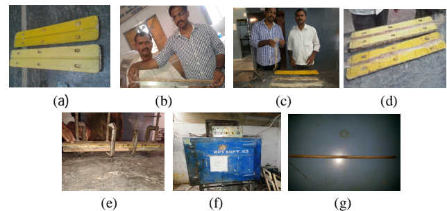
Fig 2. (a): Mould for the preparation of Wear Test ASTM Standards. Fig (b): Measuring and cutting the Fibers as per the Requirement. Fig (c): Required length of fibers for fabrication. Fig (d): Applying Epoxy Resin, Hardener & Fiber layer by layer. Fig (e): Both Pieces of mould attached and applying the C-Clamps. Fig (f): Furnace for Annealing Process. Fig (g): Full length Fabricated Specimen.
