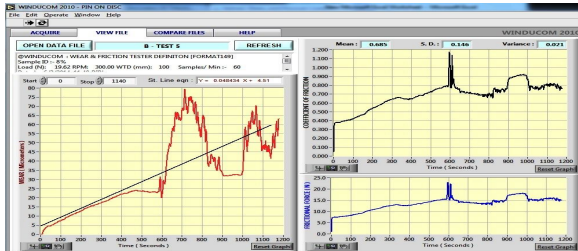
Fig 11 Graph for Wear, Coefficient of friction, friction force for 24% HNFPCM for 20N.
