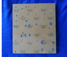
The basement board was drilled by a driller. On the basement board many circuits should be placed and is to be mounted with a screw. For inserting the screw we should drill some hole on the board as shown on the board. The basement board holds all the electrical parts and circuits.
