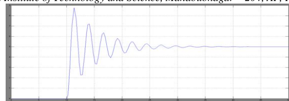
Fig 9: Response of dc motor with P-Controller
