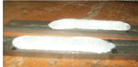
Fig 4: After coating of aluminium over mild steel the formation of layers along the plate
