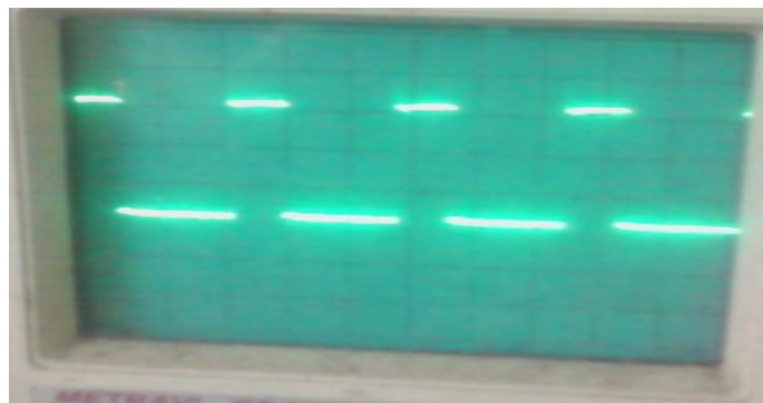
Figure14. Transformer secondary voltage T(s)
