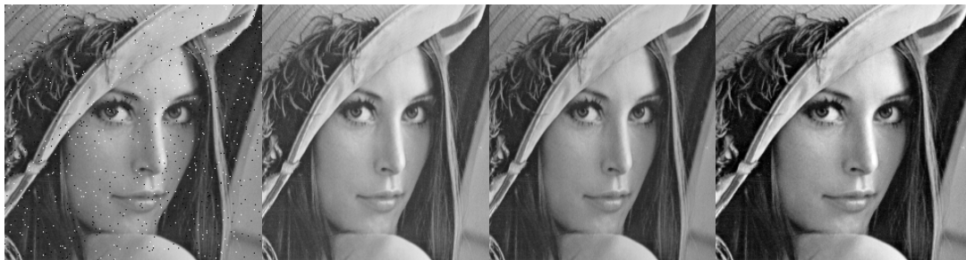
Fig. 9 Visual quality comparison of the proposed method tested with Lena gray scale image of size 128 x 128. From left to right: low resolution input with noise, Bilinear, SWT/DWT, proposed method output.
