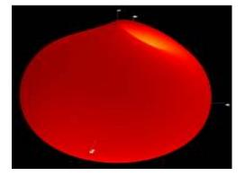
Figure 8  $E_{\varphi}$  (dB) measured radiation patterns at 5.8312 Ghz Radiation efficiency
