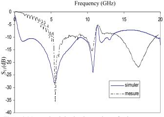
Figure.4. Measured and simulated return losses for the antenna.
