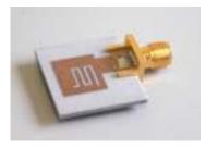
Figure. 2. UWB antenna prototype
