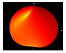
Figure 5:  $E_{\theta}$  (dB) measured radiation patterns at 4.7566 Ghz
