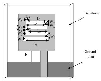
Figure.1 : Geometry of the antenna.
