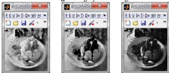
Red component Green component Blue component Figure 8. Separation of Red,Green and Blue component
