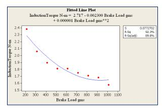
Fig 9: Fitted Line plot for Input disk torque
