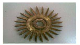
Fig 5. Impeller of pump and turbine
