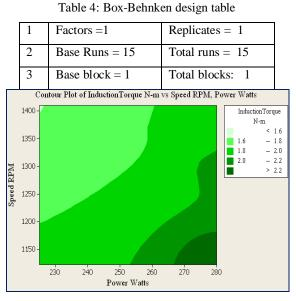
Fig 8: Contour plots of Input disk torque
