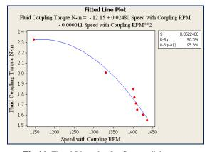
**Fig 11:** Fitted Line plot for Output disk torque **Table 5:** Coefficients of Regression equation obtained
