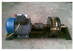
Fig 2. Induction motor with fluid coupling
