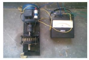
Fig 4. Wattmeter connected to motor
