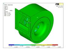
4.2.1Displacement of composite blower in x-y-z-direction, mm  $\,$
